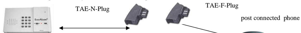
1. Plug adapter TAE-N into first N-Jack of wall plate
