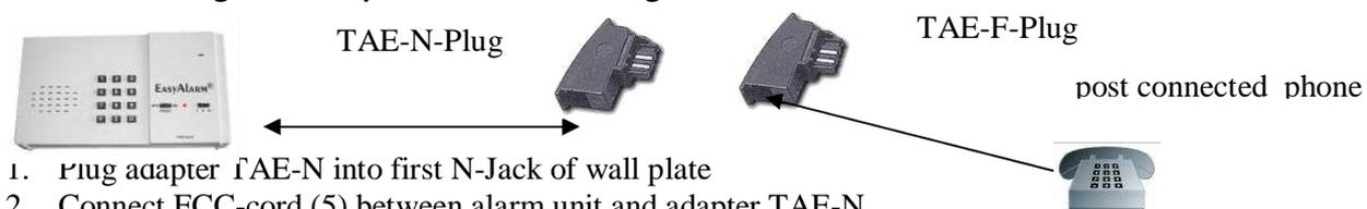
1. Plug adapter TAE-N into first N-Jack of wall plate
